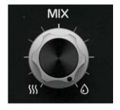
The MIX knob controls the blend of the WET signal and the DRY signal.
