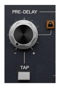
PRE-DELAY is the time between the end of the initial sound and the beginning of the first reflections being audible, hence unmasking the initial attack allowing it to cut through the mix. By adjusting the pre-delay time, you can achieve a balance that enhances spatial characteristics without compromising the clarity and definition of the source sound.
