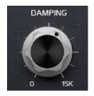
DAMPING emulates the mechanical mechanism used in plate reverbs to absorb high frequency content in the reverberated signal. All frequencies above the chosen frequency are subject to absorption.
