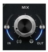
The MIX knob controls the blend of PLATE REVERB processed and incoming signals. Incoming signal is defined by the position of the Plate when the modules are set in series:
