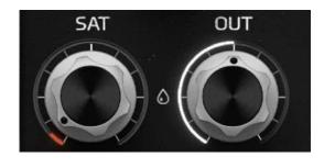
SAT applies P42 saturation to the signal arriving at the OUTPUT module. Saturation applies to the WET signal; **it is not applied to the dry signal**.
