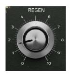
The REGEN knob controls the number of times a portion of the delayed signal is fed back into the beginning of the delay line. Setting this dial to a value of 8 or above will achieve a runaway effect. This effect requires caution because the output level will continue to increase to the point of internal clipping.
