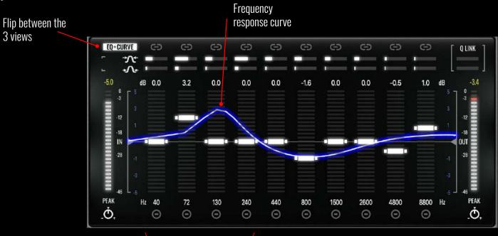
low-frequency bands are close together—so the curve display doesn't always pass exactly through every slider point
