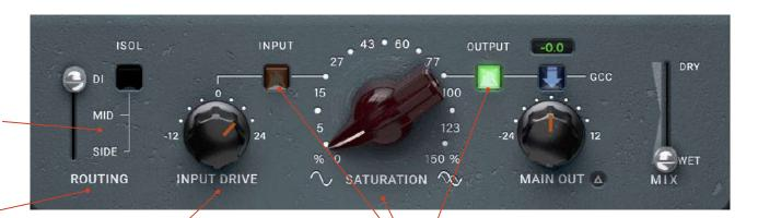
Switches processing between mono/stereo (DI), mid (MID) or side (SIDE).
