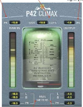
RAW RMS signal for left, right channel and peak.
