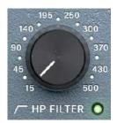
Signature 12 dB/oct HPF. Use in tandem with the low shelf to influence the focus, weight and warmth of the low end of any signal.
