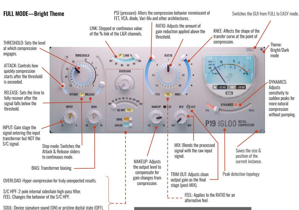
Hold the shift key when adjusting the INPUT IN to compensate equally with the MAKEUP knob.
