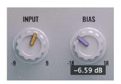
**INPUT:** Controls the gain feeding the input transformer. Lower settings keep the signal cleaner, while higher settings increase harmonic coloration, shaping the tone before compression. This gain does not affect the sidechain signal—it's purely for tone.
