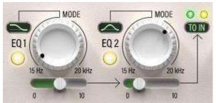
Two multi- functional EQ bands can be used to simultaneously alter the signal sent to the detector circuit (TO SC) and to alter the signal sent through the processing chain prior to
