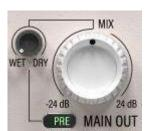
The MAIN OUT knob features -24 dB to 24 dB of clean gain.
