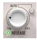
RELEASE controls the time it takes to fully recover back to the unaffected gain level once the signal falls below the threshold. If AUTO is engaged, the release time is continuously and dynamically determined by Abyss. The speed of the program dependent release time can be influenced by adjusting the RELEASE knob.
