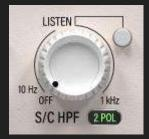
S/C HPF applies a high-pass filter to the detector circuit. This filter does not directly affect the sound of the processed signal. The slope of the HPF can be adjusted using the 1 POL / 2 POL switch to the right of the S/C HPF label. The 1 POL option gives a 6
