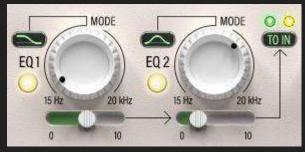
Two multi- functional EQ bands can be used to simultaneously alter the signal sent to the detector circuit (TO SC) and to alter the signal sent through the processing chain prior to
