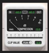
The dB COMPRESSION gain reduction meter main window shows the RMS (Root-Mean-Square) gain reduction applied to the signal as indicated by the ballistic needle. To the right of the needle is a display box that
