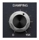
DAMPING emulates the mechanical mechanism used in plate reverbs to absorb high frequency content in the reverberated signal. All frequencies above the chosen frequency are subject to absorption.
