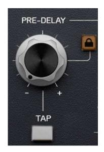
PRE-DELAY is the time between the end of the initial sound and the beginning of the first reflections being audible, hence unmasking the initial attack allowing it to cut through the mix. By adjusting the pre-delay time, you can achieve a balance that enhances spatial characteristics without compromising the clarity and definition of the source sound.
