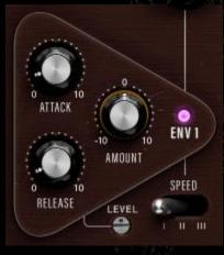
The envelope follower extends the filtering capabilities of either the cutoff frequency, resonance and slope or the NOTCH/PEAK band filter, turning these into dynamic filters.
