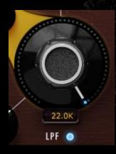
The LPF cutoff frequency knob sets the point from where the low pass filter starts working.
