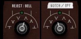
The switchable NOTCH/PEAK band filter selector allows for choice from three notch filters and three bandpass peak
