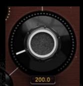
The NOTCH/PEAK band filter frequency knob sets the center point of the selected filter.
