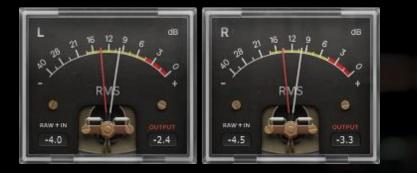
The P455 VU meters provide a nuanced representation of perceived loudness by presenting the average input and output levels calculated over a brief period (RMS). Peak dBFS values are shown in the lower quadrants of the meters.
