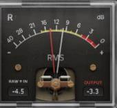
The P455 VU meters provide a nuanced representation of perceived loudness by presenting the average input and output levels calculated over a brief period (RMS). Peak dBFS values are shown in the lower quadrants of the meters.
