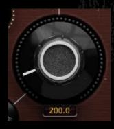
The NOTCH/PEAK band filter frequency knob sets the center point of the selected filter.
