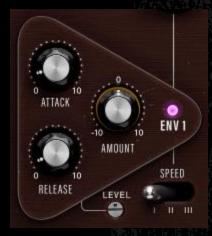
The envelope follower extends the filtering capabilities of either the cutoff frequency, resonance and slope or the NOTCH/PEAK band filter, turning these into dynamic filters.
