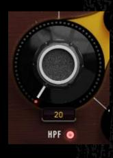
The HPF cutoff frequency knob sets the point from where the high pass filter starts working.
