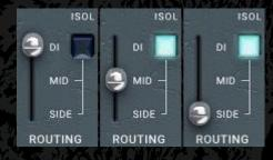
Switches processing between mono / stereo (DI), mid (MID) or side (SIDE). The mid and side options are only available when the plugin detects a stereo signal.
