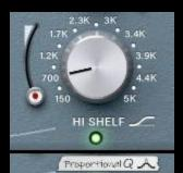
The switchable HI SHELF / Proportional Q Bell filter allows for flexible choice of filter type. Click on the HI SHELF or Proportional Q label to switch between these options
