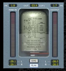
The metering shows several pieces of information including LUFS (Loudness Units relative to Full Scale) measurements, dBFS PK (decibels relative to full scale peak hold) measurements, and switchable RMS / PEAK RMS (Root-Mean-Square) bar meters and measurements.
