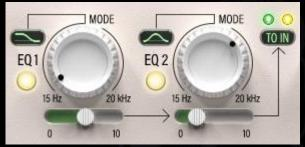
Two multifunctional EQ bands can be used to simultaneously alter the signal sent to the detector circuit
