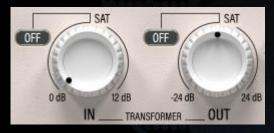
The T. IN and T. OUT gain knobs provide either pristine digitally clean or mojo infused transformer coupled amplifiers for adjusting gain pre and post
