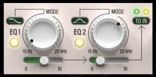
Two multifunctional EQ bands can be used to simultaneously alter the signal sent to the detector circuit
