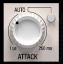
ATTACK controls the time it takes to fully reach the target gain adjustment based on the threshold and ratio settings.
