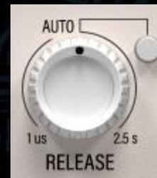
RELEASE controls the time it takes to fully recover back to the unaffected gain level once the signal falls below the threshold.
