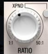
RATIO Determines the amount by which to adjust gain, and hence dynamic range, once the signal has passed the threshold.
