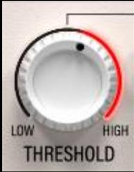
Sets the level at which gain adjustment is applied.
