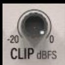
None shall pass. The CLIP knob sets the dBFS (decibels relative to full scale) RMS value at which the analog clipper hard clips the signal with beautifully transparent, pristine quality clipping. As with real-world imperfect analog clipper circuits, overshoots can sometimes occur randomly within a +0.3 dB tolerance. 'Tis but a scratch.
