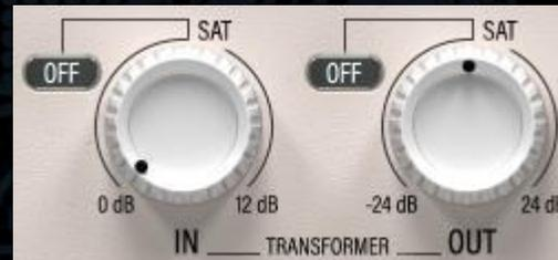
The IN and OUT gain knobs provide either pristine digitally clean or mojo infused transformer coupled amplifiers for adjusting gain pre and post
