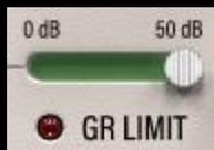
Limits the maximum gain reduction to the specified value. Without this set, the compressor or expander/gate will apply gain reduction as determined by the ratio and threshold without restrictions. With this set, the gain reduction will not exceed this value.
