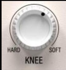
The KNEE influences the abruptness of the gain adjustment at the time the threshold is crossed. This is most easily influenced by imagining a sharp angle at the HARD position, gradually transitioning to a rounded curve at the SOFT position.
