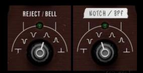
The switchable NOTCH/PEAK band filter selector allows for choice from three notch filters and three bandpass peak filters.
