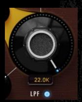
The LPF cutoff frequency knob sets the point from where the low pass filter starts working.
