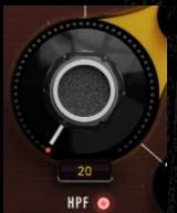
The HPF cutoff frequency knob sets the point from where the high pass filter starts working.
