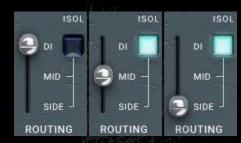
Switches processing between mono / stereo (DI), mid (MID) or side (SIDE). The mid and side options are only available when the plugin detects a stereo signal.
