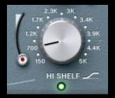
The high shelf filter shares a similar advanced filter topology to that of the low shelf filter and features an ultra-smooth boost that ranges from 150 Hz to 5 kHz. The boost slider ranges in intensity from 0 to 10.
