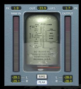
The metering shows several pieces of information including LUFS (Loudness Units relative to Full Scale) measurements, dBFS PK (decibels relative to full scale peak hold) measurements, and switchable RMS / PEAK RMS (Root-Mean-Square) bar meters and measurements. The PK (peak hold) measurements hold the highest measured value. They will be reset if any measurements are clicked, if the DAW is stopped/started or if the Meter Reset button adjacent to the MAIN OUT label is clicked.
