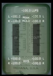
The metering HUD (heads up display) show several pieces of information including LUFS (Loudness Units relative to Full Scale) measurements, dBFS (Decibels relative to Full Scale) PEAK HOLD measurements, and switchable RMS / PEAK RMS (Root-Mean-Square) bar meters and measurements.
