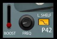
The advanced filter topology of this low shelf filter features a musical boost that ranges from 40 Hz to 5 kHz. The boosted portion of the signal is followed by a frequency dip that helps to frame the area of focus.
