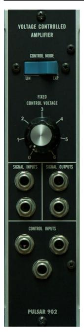
The 902 VCA has two modes, linear and exponential. Linear is normally used for the amp envelope and exponential mode is useful for CV signals.
