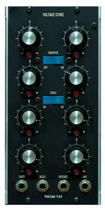
The 935 Voltage Store is a very simple 8-step voltage store. Each step is controlled by a dedicated potentiometer with an adjustable output ranging from -6 to +6 volts.
