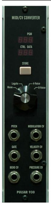
The MIDI/CV module is where all MIDI events from the host DAW get converted into (virtual) CV/Gate voltages and injected into the modular engine, which runs at the host sample rate or some multiple thereof when oversampled. Smoothing filters are used where needed to avoid audible steps when generating high resolution control voltages from (course) MIDI data.
