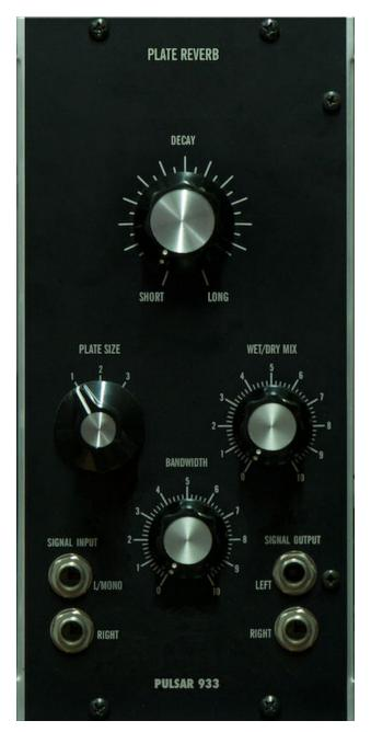
The 933 Plate Reverb is using a reverberation network topology similar to those used in high end early 1980s digital effects processors, with modulated tails. It is a very good sounding and flexible reverberation algorithm for which 3 different plate size configurations are provided.
