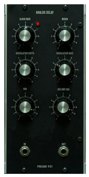
The 931 Analog Delay is an emulation of a Bucket Brigade Delay (BBD) - a discrete-time analog delay line popular in the 1970s and the early 1980s. The emulation includes the filtering, distortion and noise typical of such delays. The BBD control allows the distortion and noise part of the emulation to be mixed in as desired. When fully attenuated you have a clean delay that can be just as useful as the BBD distortion that provides an interesting color.
