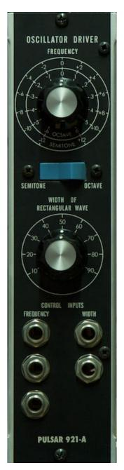
As with hardware modules, the 921-A oscillator driver has a hidden internal connection to each 921-B oscillator. It contains an exponential converter that controls the base pitch and also the pulse width of all connected oscillators.
