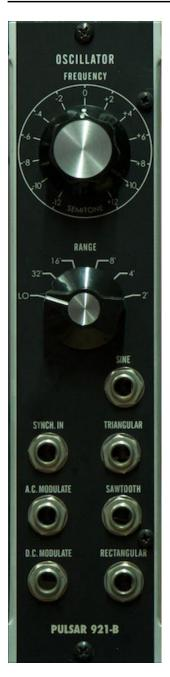
The 921-B oscillator's frequency control allows modifying the base pitch by +- 12 semitones.
