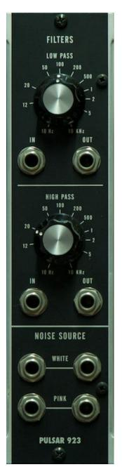
The 923 module has two 1-pole non-resonant filters. Both the low pass and the high pass filter has a cutoff range from 10 Hz to 10 Khz.
