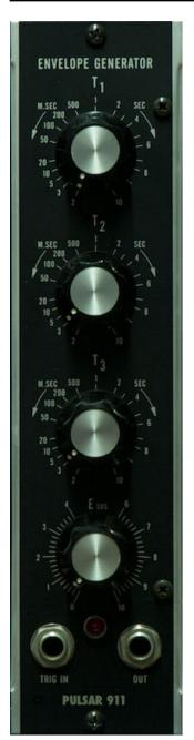
The 911 envelope generator has a general shape matching the analog equivalent, however the Pulsar version has modified timings with an attack rate closer to that of the Minimoog (which the author happens to like better). Some hard pluck sounds included in the factory presets could not be done without it.
