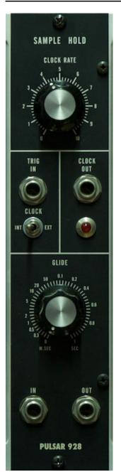
The 928 S&H module samples the input and outputs (a held value) at the rate of either the internal clock or an external clock.
