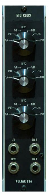
The 936 MIDI Clock uses the DAW host to generate synchronized quarter-note clock signals. In addition the module also has three independent clock dividers, each with its own output. Plus a forth output for quarter-note clock output only. The clock signals can be used to drive the 935 Voltage Store, for DAW synchronized sequences.
