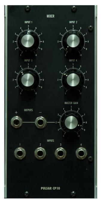
The CP10 is a "clean" mixer. It will not clip or saturate and has a gain of 6 dB. It can be used to mix either A/C or D/C signals.
