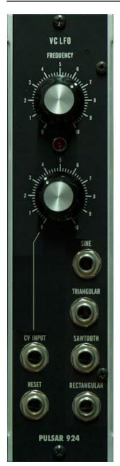
Original Pulsar module. It outputs 4 different wave forms and features CV control of the LFO frequency. The LFO frequency ranges from 0.1 to 80 Herz. The CV input control attenuates the CV signal.
