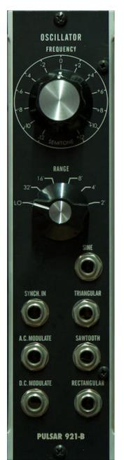
The 921-B oscillator's frequency control allows modifying the base pitch by +- 12 semitones.
