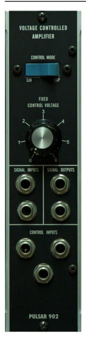
The 902 VCA has two modes, linear and exponential. Linear is normally used for the amp envelope and exponential mode is useful for CV signals.
