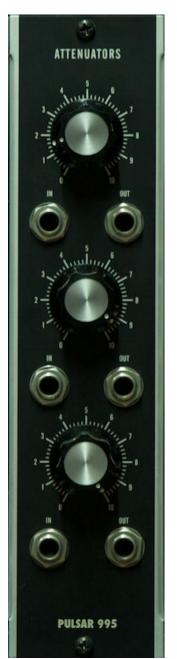
As in the original hardware, the 995 attenuator is internally connected from top to bottom. With only the first input connected, each output is active and can have different gain settings.
