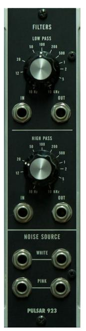
The 923 module has two 1-pole non-resonant filters. Both the low pass and the high pass filters have a cutoff range from 10 Hz to 10 Khz.
