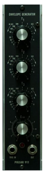
The 911 envelope generator has a general shape matching its analog equivalent. However, the Pulsar version has modified timings with an attack rate closer to that of the Minimoog (which the author happens to like better). Some hard pluck sounds included in the factory presets could not be done without it.
