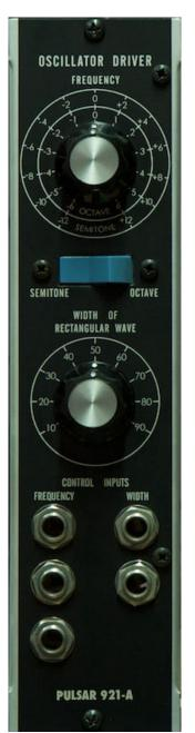
As with hardware modules, the 921-A oscillator driver has a hidden internal connection to each 921-B oscillator. It contains an exponential converter that controls the base pitch and also the pulse width of all connected oscillators.
